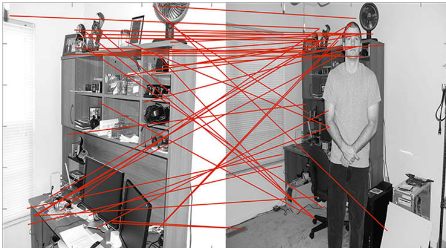
Figure 7. SURF image showing reduced keypoint matches with occlusion.
